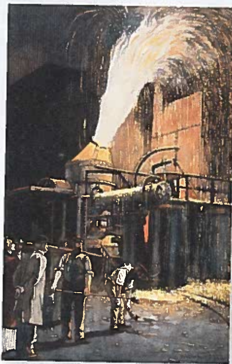
A Bessemer furnace changed molten iron into steel by forcing air through the iron to burn away carbon and other impurities.
