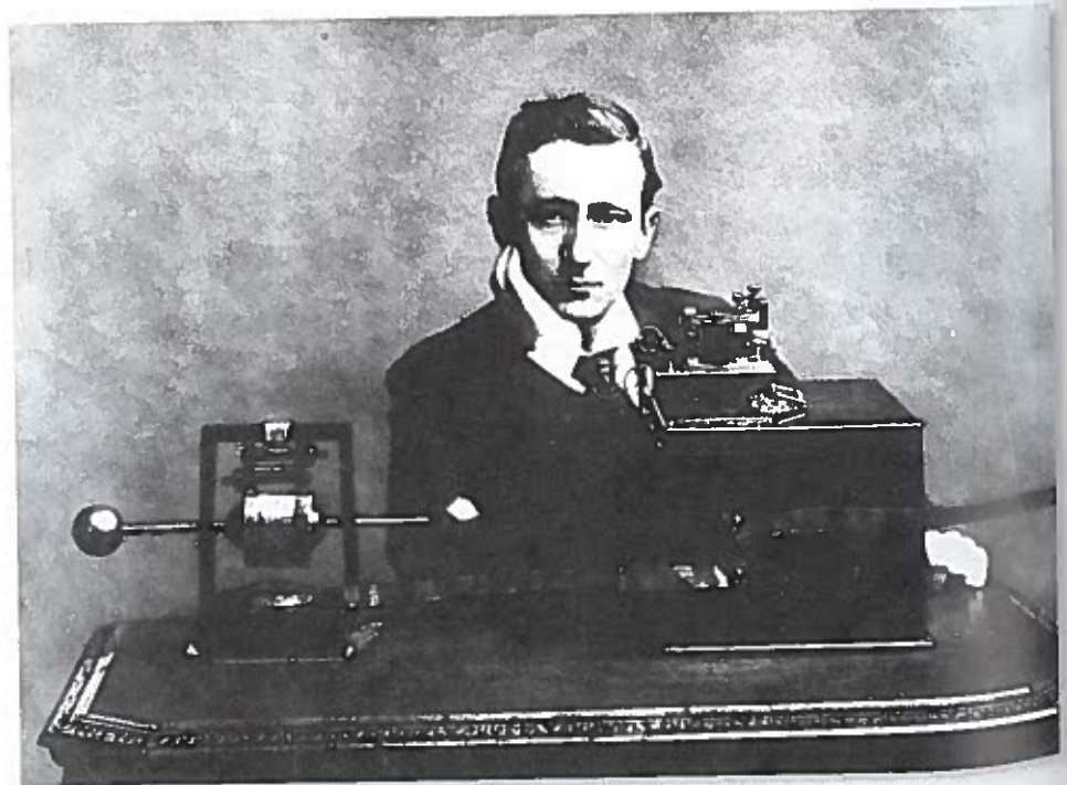
Italian electrical engineer and inventor Guglielmo Marconi is shown here in 1896 with his wireless telegraph machine.
